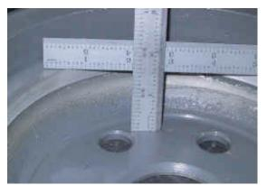
• First, measure the height from the inside of the flywheel where it touches the crankshaft flange to the surface that has the magnets installed.
