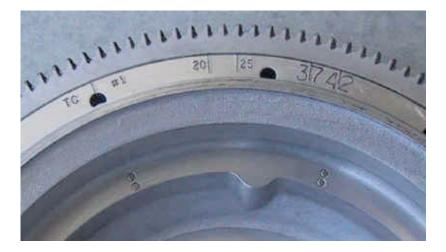
Large diameter alternator pulley required (8.5" ID).
