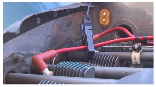
Connect the strobe light to power. Only use a simple strobe light that does not have a potentiometer or display.
